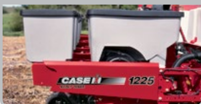
GRANULAR CHEMICAL HOPPER
