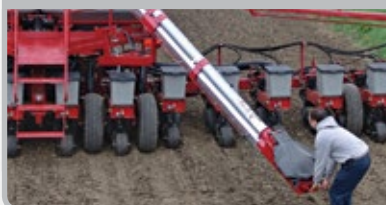
BULK FILL CONVEYOR SYSTEM
