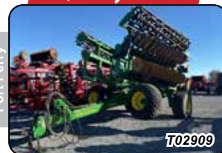
Speed Disk, John Deere 2680H, 25ft, Notched Fronts, Smooth Rears, Cage Roller, Cat 4 Hitch
