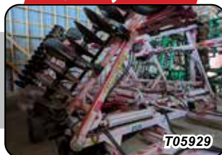
Disk, Sunflower 1444-36ft, 8.5" Spacing, Rock Flex, 23" Blades, Single Point Depth Control, Walk Tandem Wings
