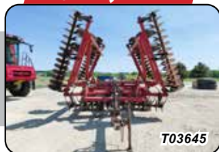
Disk, Case IH 3950-30ft, 7" Spacing, Walk Tandem Mains/Wings, Scrapers, Lights
