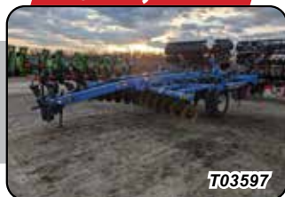
Disc Ripper, DMI Ecolotiger 730B-18ft, 7 Shank, Spring Shank Reset, 30" Spacing, Rear Leveller Discs
