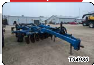
Disc Ripper, DMI Ecolotiger 530B-14ft, 9 Shank, Spring Shank Reset, 30" Spacing, Rear Level Discs
