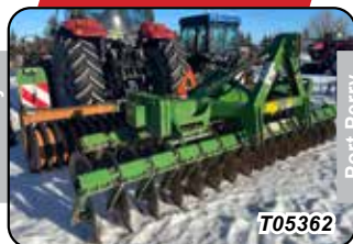
Speed Disk, Amazone Catros 4001-13pt, Dual Gang Individual Disks, Rubber Fronts, Notched Rears, Rubber Roller, Packer, Extra Weights Added
