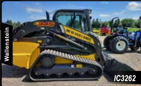
New Holland C345 Track Loader Enhanced High flow w/ride control, 84" LPE bucket & cutting edge
